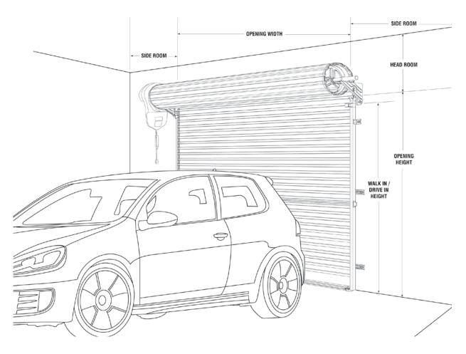
Initially invented by B&D back in the 50s, Rolling garage doors are commonly considered as amongst the most economical and functional garage doors available in Australia. Being constructed from corrugated steel they also provide strength against impacts..
